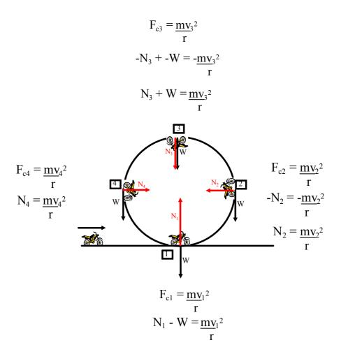
Riders must have at least a minimum speed at the top of the circle to remain on the track. This speed can be determined by considering the centripetal force at point 3. The  $v_3$  is a minimum when  $N_3$  is zero. At this speed the track does not exert a normal force to keep the motorcycle on the path because the weight provides all of the centripetal force. The rider experiences apparent weightlessness - rider and motorcycle are falling freely toward the center of the circle.
