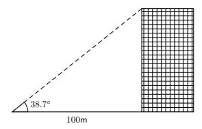
Figure 15.1: Determining the height of a building using trigonometry.
