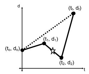
$$v_{\mathbf{x}} = slope = \frac{d_2 - d_1}{t_2 - t_1} = \frac{\Delta d}{\Delta t}$$
