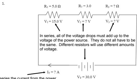
In series the current from the power source goes through each resistor.
