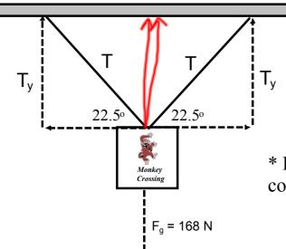
A sign that weighs 168 N is supported by two ropes, A and B, that make 22.5° angles with the horizontal. Determine the tension along the ropes.
