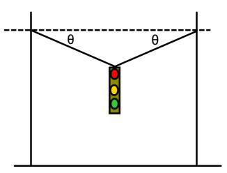
A traffic light is to be hung like in the diagram to the right. The cable being used will break if its tension reaches 1750 N. What is the largest mass that can be hung? (Answer: 151 kg)
