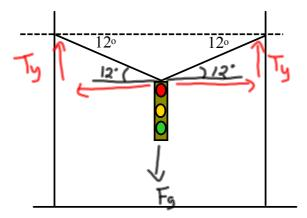
A traffic light hangs in the center of the road from cables as shown in the figure. (a) If the mass of the traffic light is 65 kg, what is the magnitude of the force that each cable exerts on the light to prevent it from falling? (b) What is the tension in each cable?
