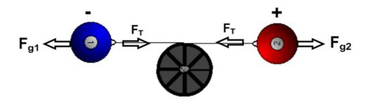
Calculate the acceleration of the connected masses of an Atwood machine that has a 15 kg mass on one side and 24 kg on the other.
