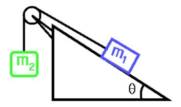
A counterweight is used to slide an object up an inclined plane that makes a 42° angle with the horizontal. The counterweight has a mass of 40 kg and is suspended with a massless string and a friction less pulley. The coefficient of kinetic friction on the plane is 0.33. For the acceleration of the object not to exceed 0.22 m/s up the ramp, what must be the minimum mass of the object?
