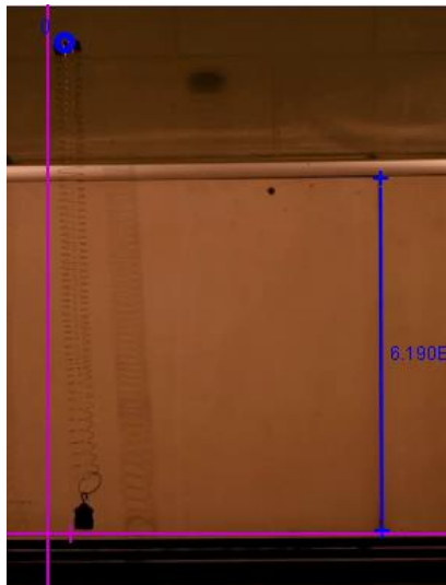
Figure 3: Similar to Figure 2, but with the 1.0 kg mass attached to the bottom of the slinky. Note the longer stretch length at that the mass is a few inches above the floor.
