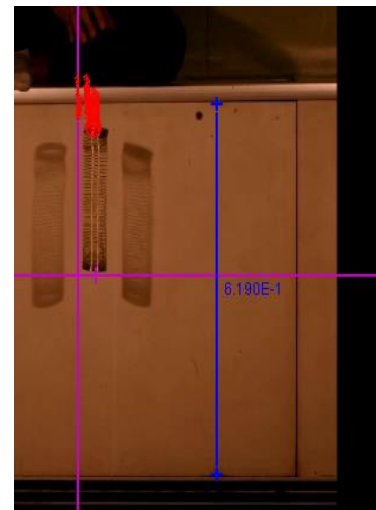
Figure 2: A screen shot from the Tracker Video Analysis program showing the coordinate system (crossed lines on the left) and the calibration stick (vertical line on the right). The markings above the slinky are the tracks made by the program.
