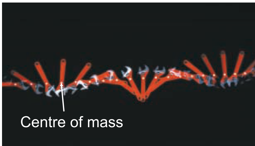
Figure 10.15 The wrench is rotating around the mark on the wrench while the mark is moving in a straight line.
