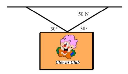
2. If the sign has a mass of 5.00 kg, what is the tension in the cables? (38 N)
