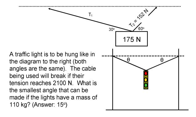
A traffic light is to be hung like in the diagram to the right. The cable being used will break if its tension reaches 1750 N. What is the largest mass that can be hung? (Answer: 151 kg)
