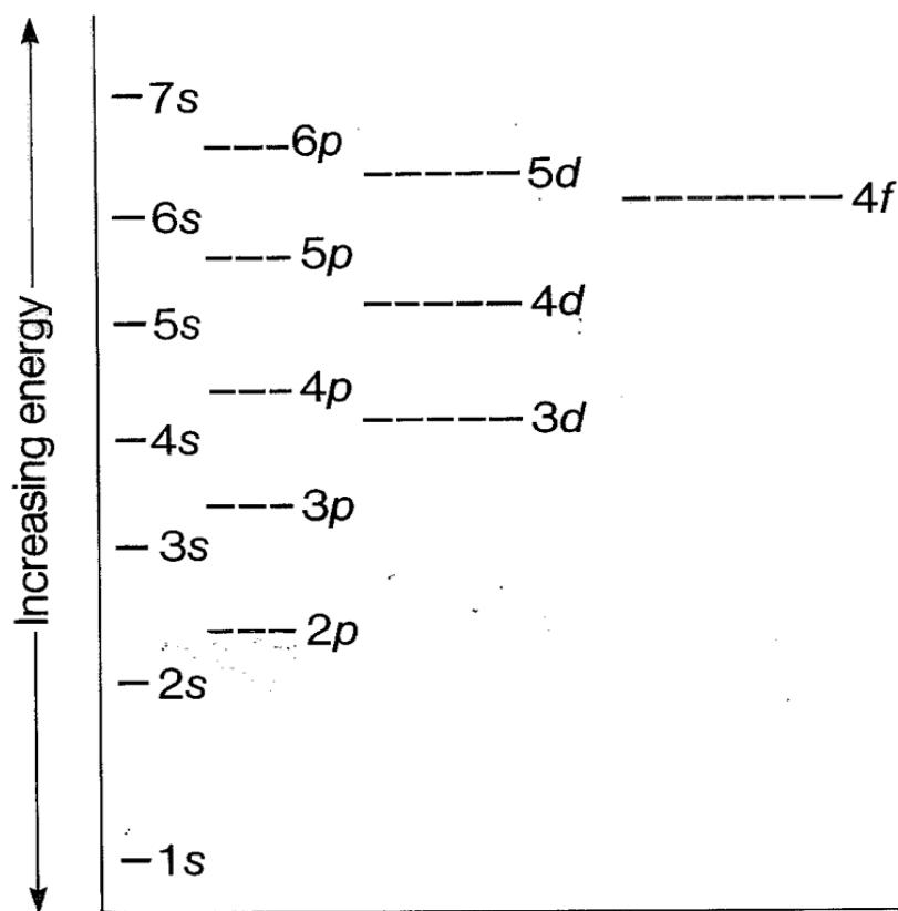
**Aufbau principle** - electrons occupy orbitals of lowest energy first
