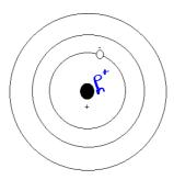
2. Electrons cannot exist between orbits, but they can move to unfilled orbits if a quantum of energy is absorbed or released.
