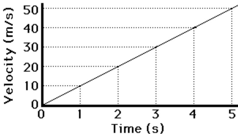
$$a = \frac{v_f - v_i}{t_2 - t_1}$$
