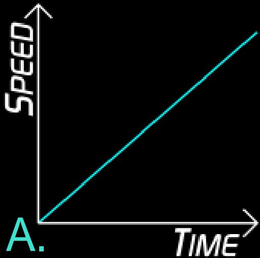
Graph A shows a constant acceleration and an increasing speed.
